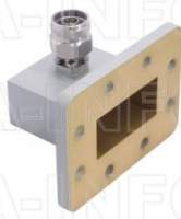
187WCANM Right Angle Rectangular Waveguide to Coaxial Adapter 3.95-5.85GHz WR187 to N Type Male
